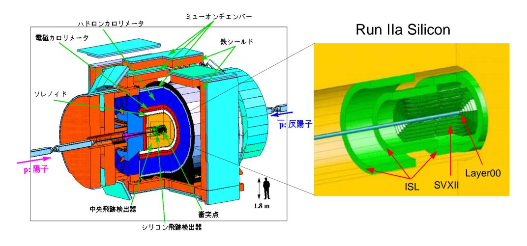
Run IIa Silicon tracker consists of Layer00(L00), SVXII, and Intermediate Silicon Layers(ISL)
