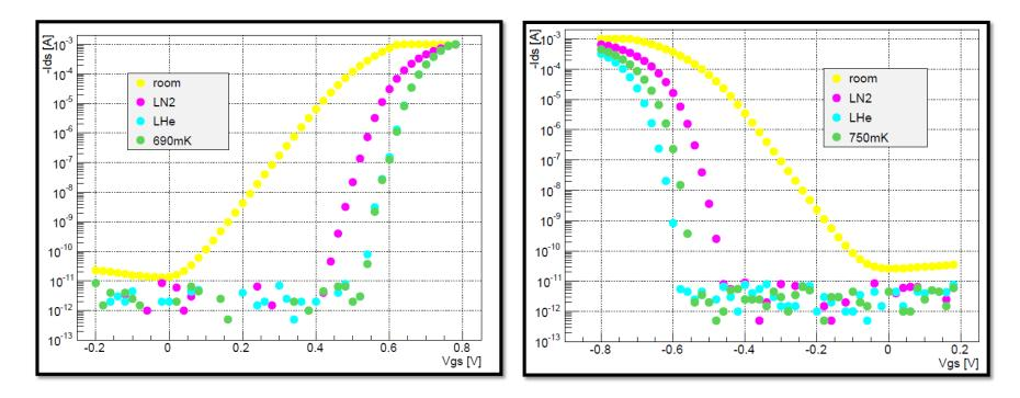
Threshold voltage is changed. But the other properties are almost unchanged.
