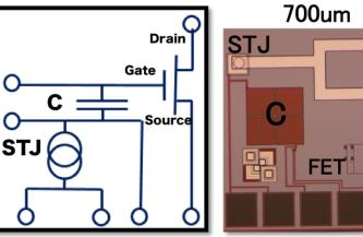
STJ processed on SOI and schematic of prototype
