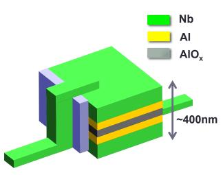
We are developing STJ photon detector for neutrino decay search (as Dr. Takeuchi slide) aiming at detecting single far infrared(50um) photon
