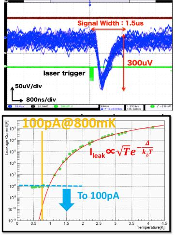
The signal to infrared(1310nm) laser Typical signal width is about 1us
