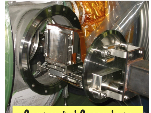
Segmented Secondary Emission Monitor (SSEM)
