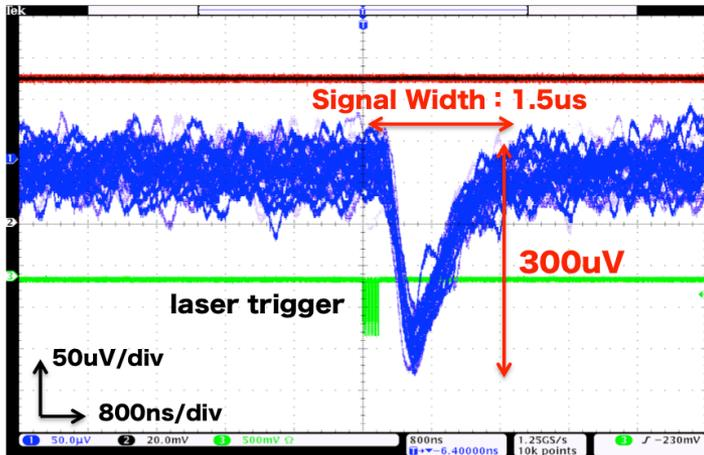
The signal to infrared(1310nm) laser
