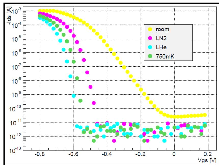
Threshold voltage is changed. But the other properties are almost unchanged.
