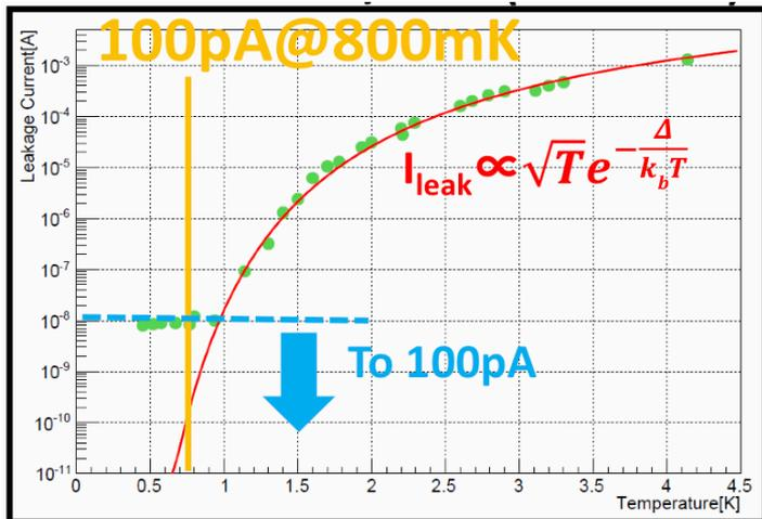
Temperature dependence of leakage current
