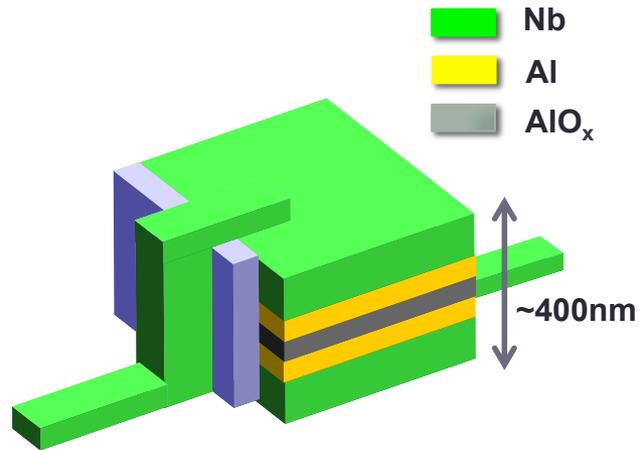
We are developing STJ photon detector for neutrino decay search (as Dr. Takeuchi slide) aiming at detecting single far infrared(50um) photon
