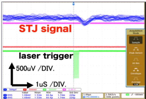
Signal of Nb/Al-STJ processed on SOI board to 465nm light
